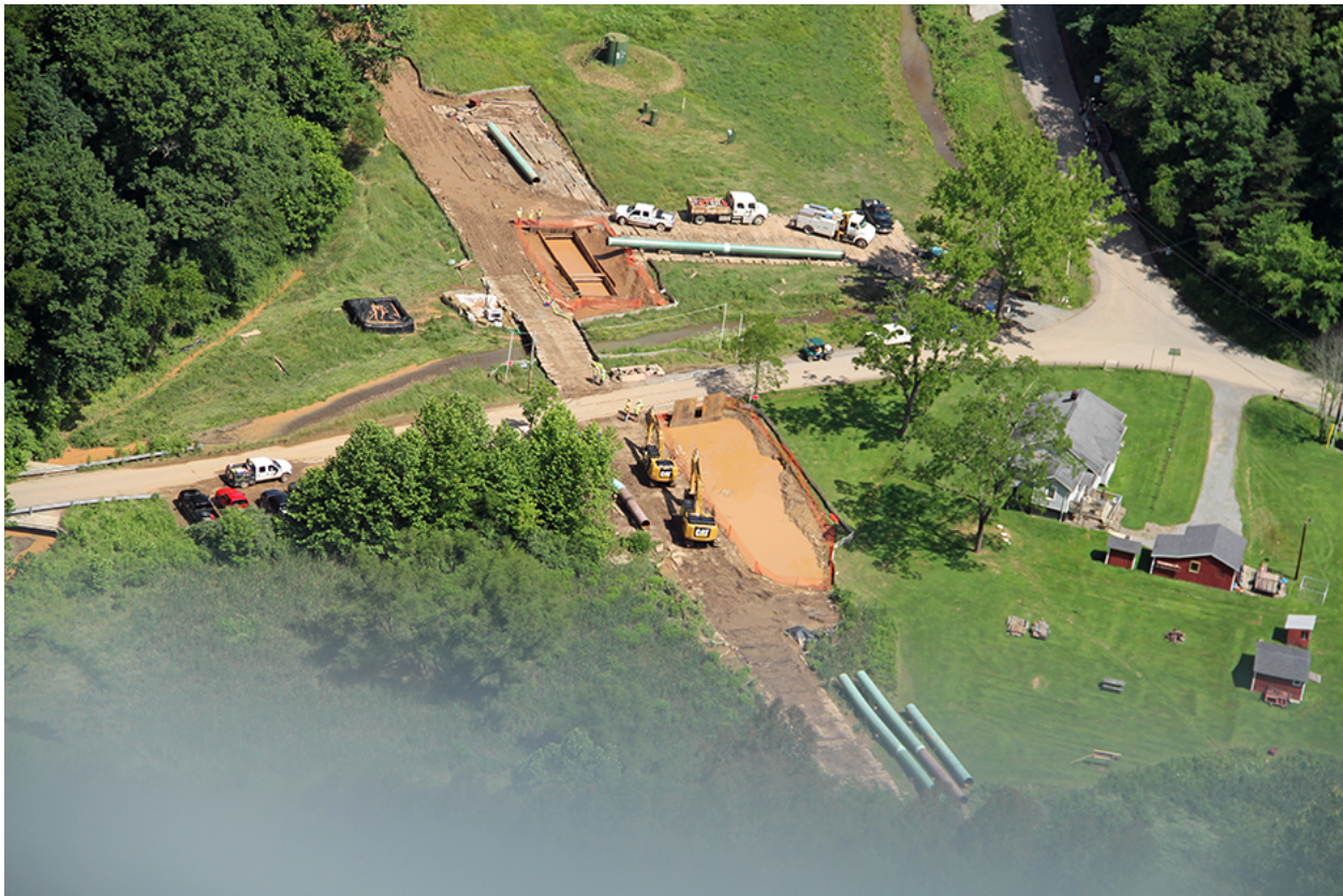
Big Isaac Creek, West Virginia: June 22, 2015. Sediment laden runoff pumped directly into stream and wetland area, bypassing sediment filtering structure, Stonewall Gathering Pipeline. Photo by Dominion Pipeline Monitoring Coalition Pipeline Air Force.
