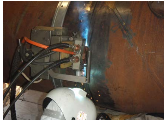
Figure 21: Automatic Welding Set up
