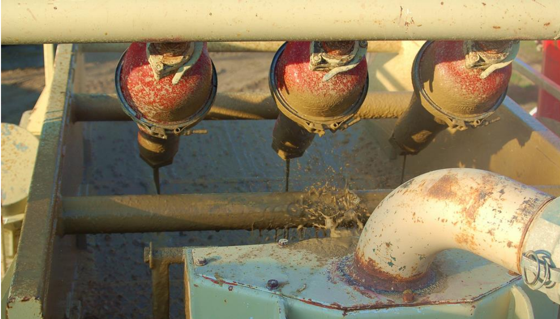
Shakers separating drilling muds and cuttings. Photo by Cowgirl Jules.
