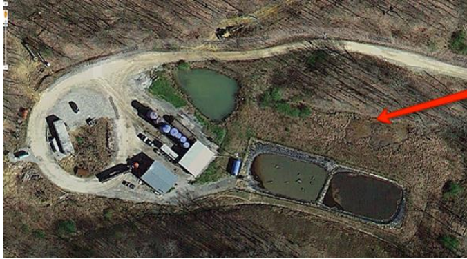
Lochgelly injection well and sediment pits in West Virginia, with seepage at the surface. Photo courtesy of DirtySecretWater.com.
