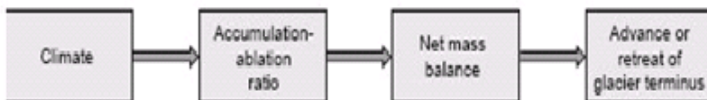
Figure 5.2.1. Relationship between and among climate, accumulation/ablation, net mass balance, and position of a glacier terminus. Adapted from Easterbrook, D.J. 1993. Glacial Processes; Surface Processes and Landforms . Prentice Hall, pp. 293–332.
