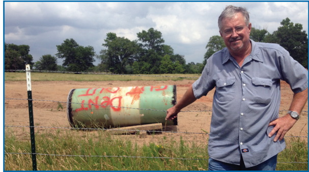
David Whitley stands near his fence with a short piece of removed pipe marked "Dent" and "Cut Out."
