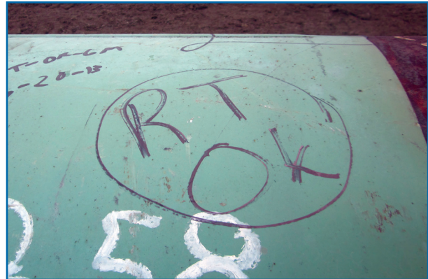
Proof that radiography testing (RT) was used during construction. This notation was seen on pipe on multiple East Texas properties.
